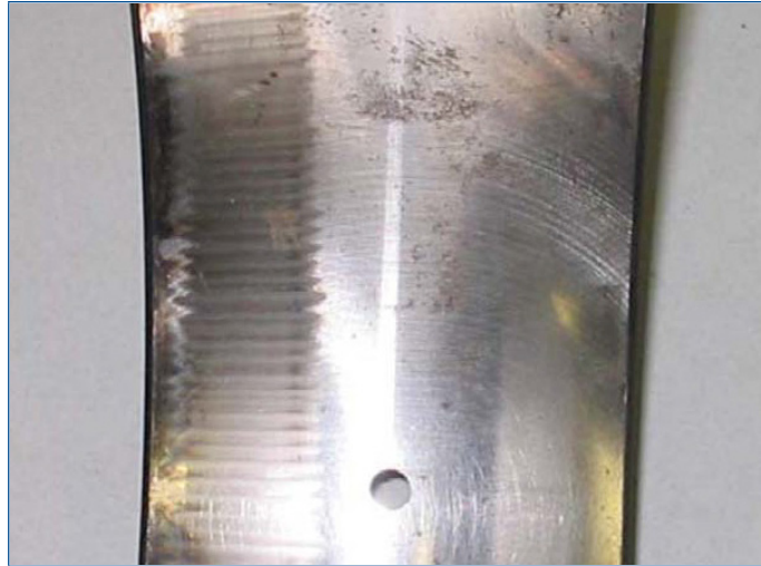
Figure 12. Defective bearing (fluting) from Pulverizer exhaust fan where data presented in Figures 10 and 11 were acquired.
