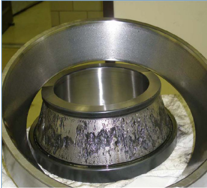
Figure 7. Photograph of the defective inner race from bearing removed from Pulverizer Gearbox following January 17, 2008 data set in Figure 6.
