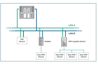
PK with Parallel Redundant Protocol (PRP) enabled in a redundant Ethernet Device Network, talking directly with native PRP devices and using a RedBox to talk to Non-native PRP devices.
