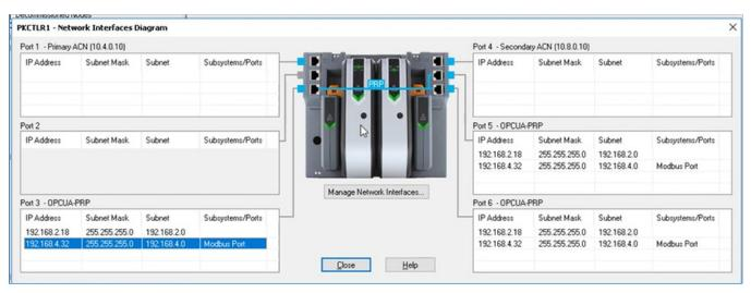
Network Interface Diagram allows you to see the network configuration for all your Ethernet ports in the PK Controller.
